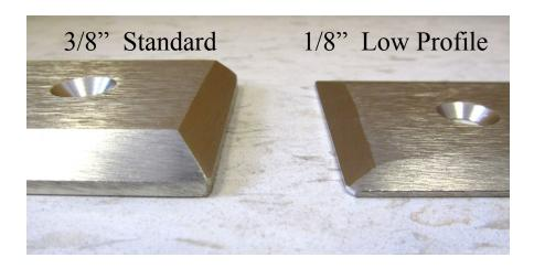
The 1/8" thick Low Profile floor plate option requires 1 extra step during installation. A shallow recessed hole in the floor, below the center hole, only 3/8" inch deep.
