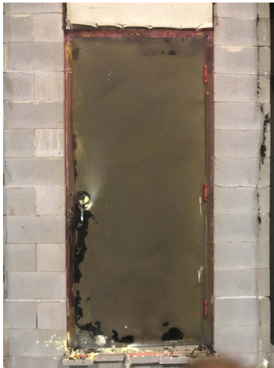
Figure 8: The exposed side of the steel door assembly after the fire test.
