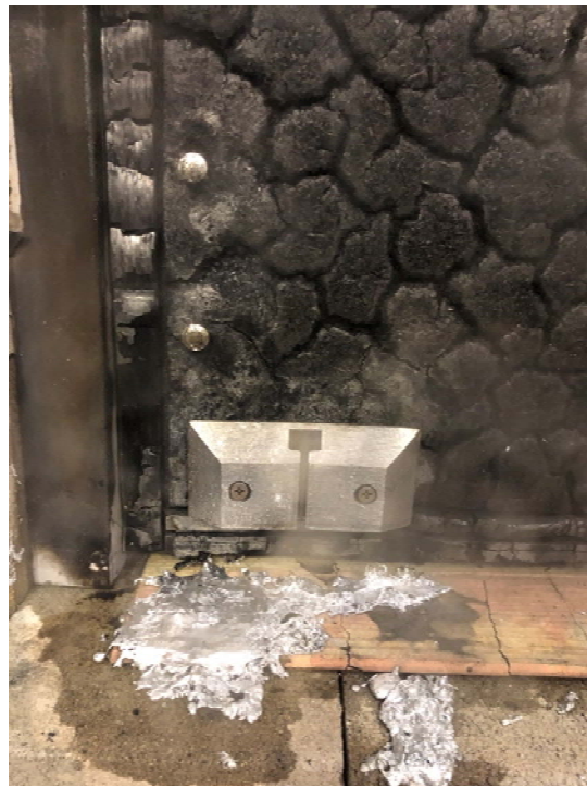
Figure 9: The exposed side of the NightLock after the hose stream test.
