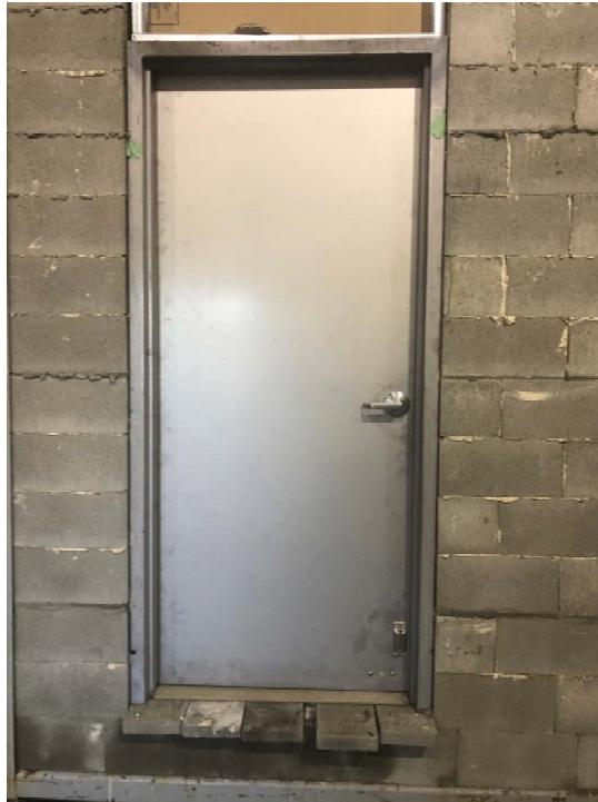
Figure 7: The unexposed face of the steel door test assembly prior to the fire test.
