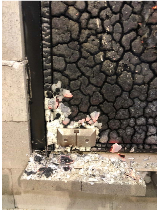
Figure 8: The exposed side of the NightLock after the fire test.
