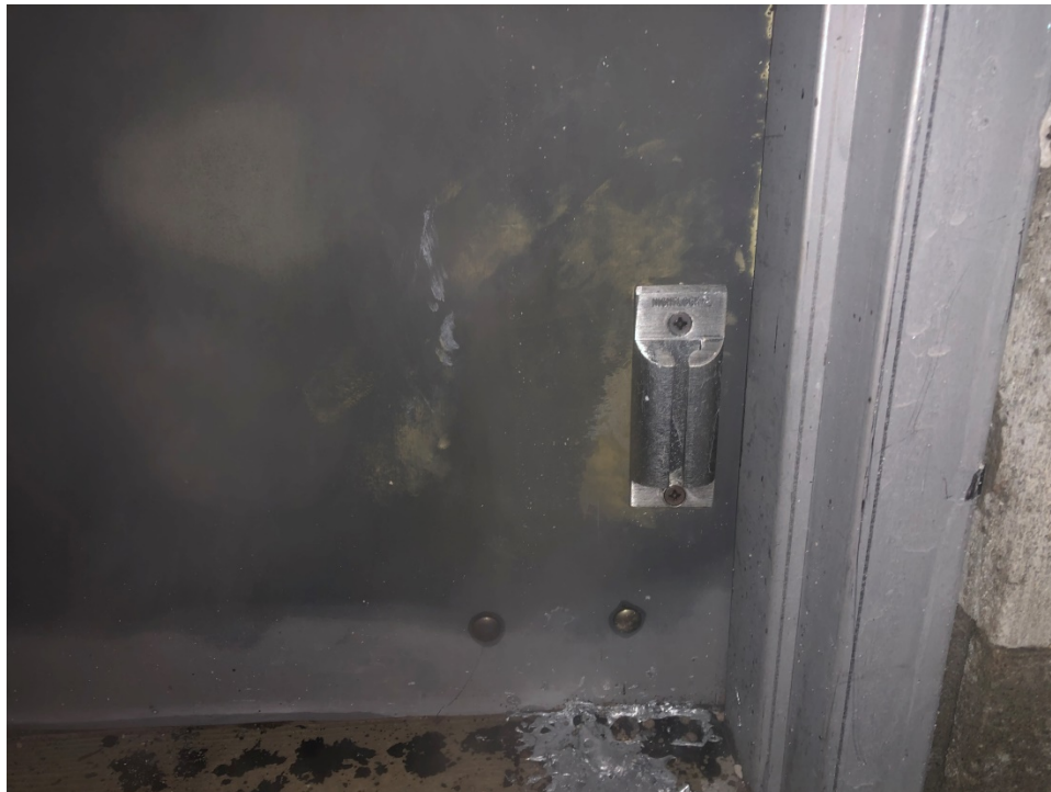
Figure 9: The unexposed side of the NightLock after the hose stream test.
