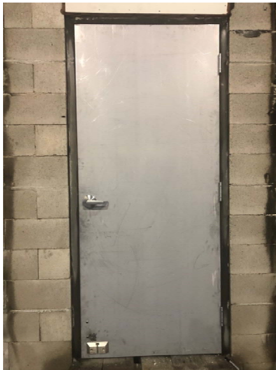
Figure 11: The exposed face of the steel door test assembly prior to the fire test.
