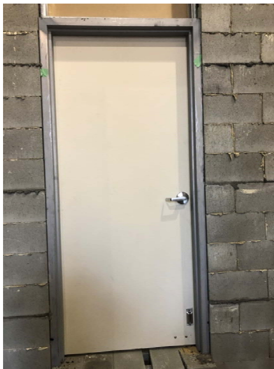
Figure 7: The unexposed face of the wood door test assembly prior to the fire test.
