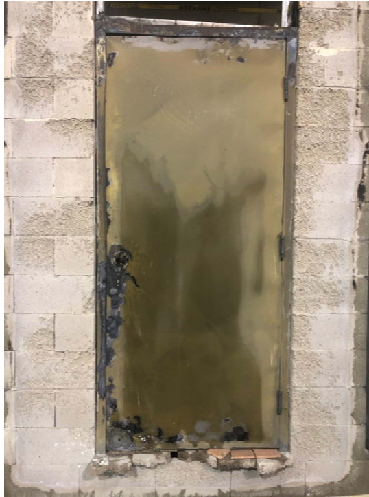
Figure 9: The exposed side of the steel door test assembly after the hose stream test.
